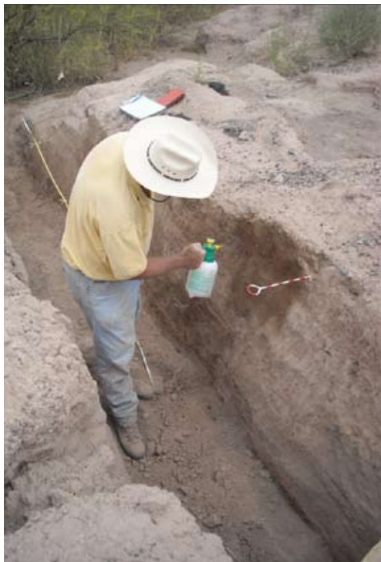
(Left) Dr. Charles Frederick wets a trench wall at the David Williams site while profiling; (right) sediments from the trench at the site are tested for texture and elasticity.
