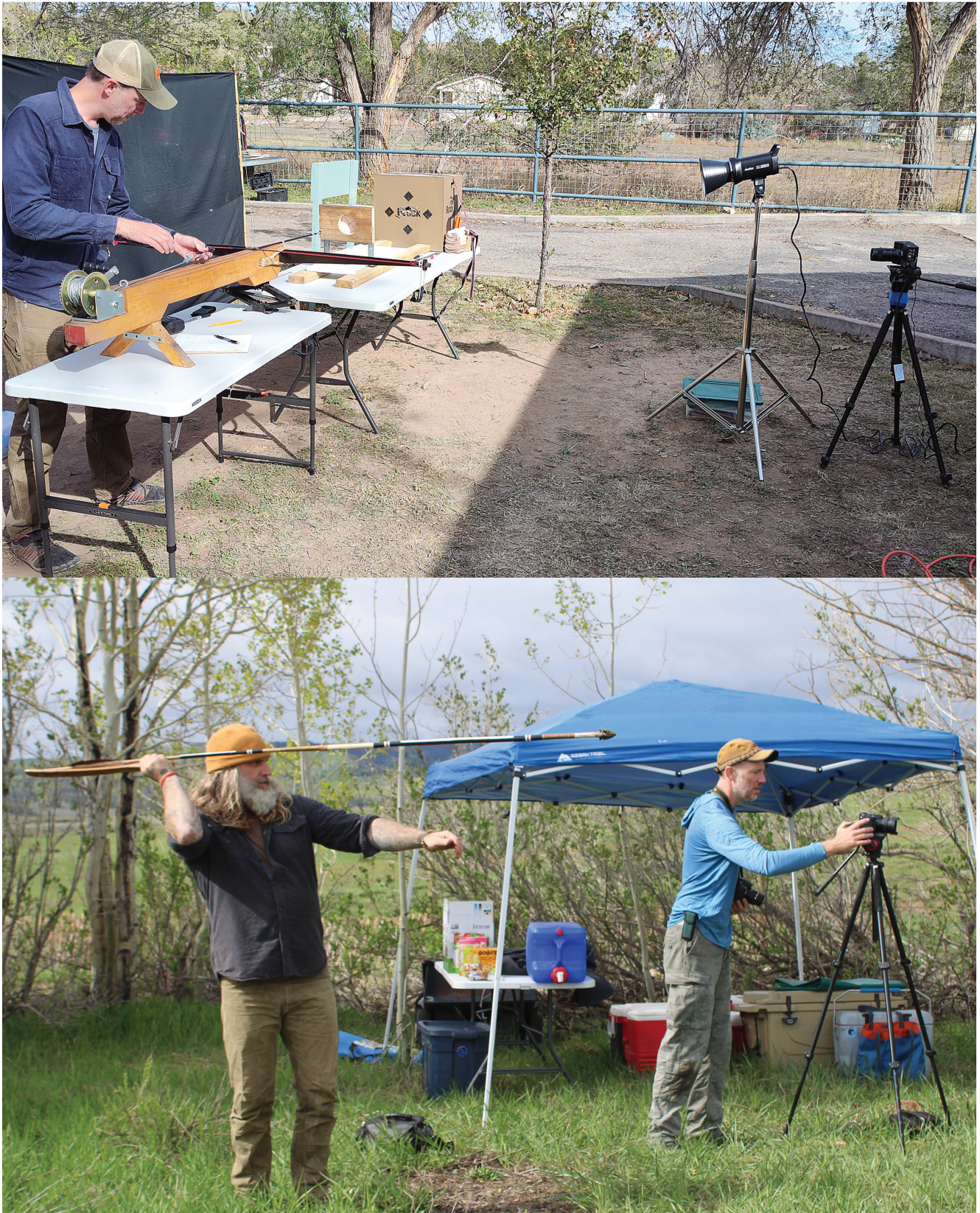
Figure 1. Example configurations of two different types of ballistic experiment; controlled (top) and naturalistic (bottom).
