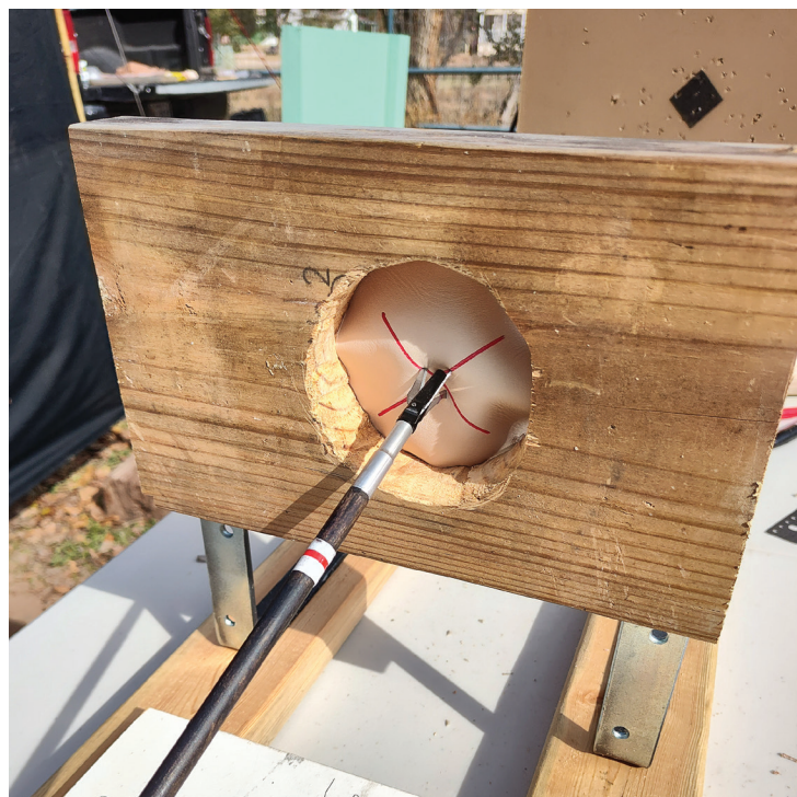
Figure 2. The result of shooting a poorly designed mechanical hunting broadhead into 2 mm thick tooling leather as a simulant for prey animal skin.
